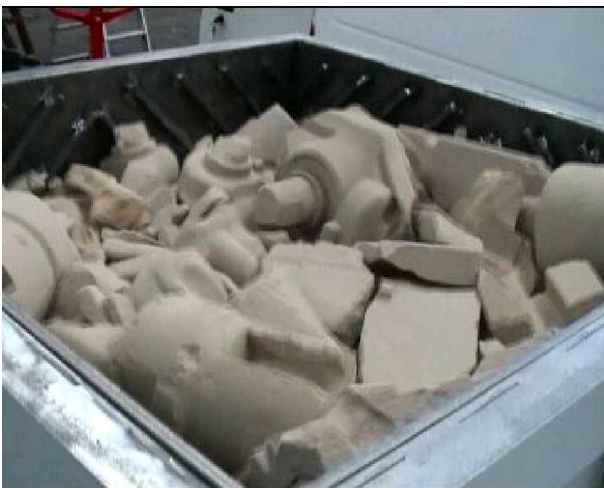
Pic.1: view into the vibrating trough with the core fraction to be recycled
