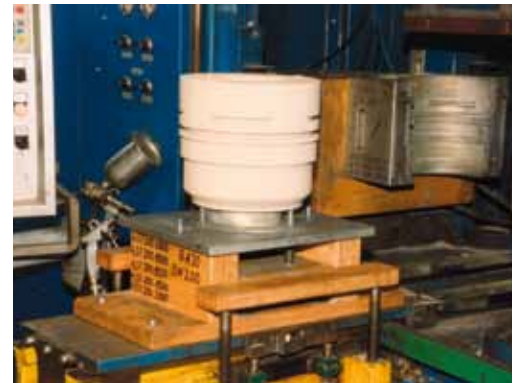
Core discharge on the machine table front
